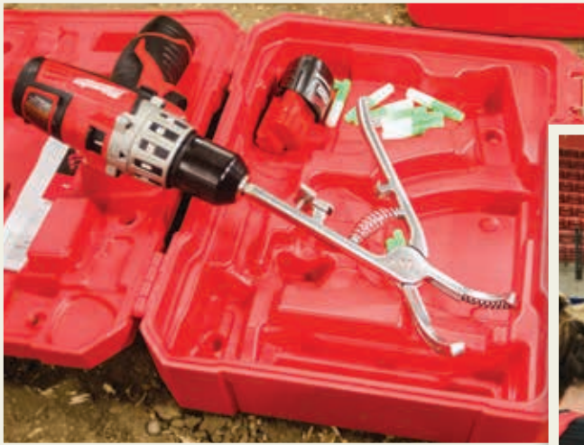
► Left: The Henderson castrator can be attached to a handheld drill and serves as a quick, bloodless castrator.
